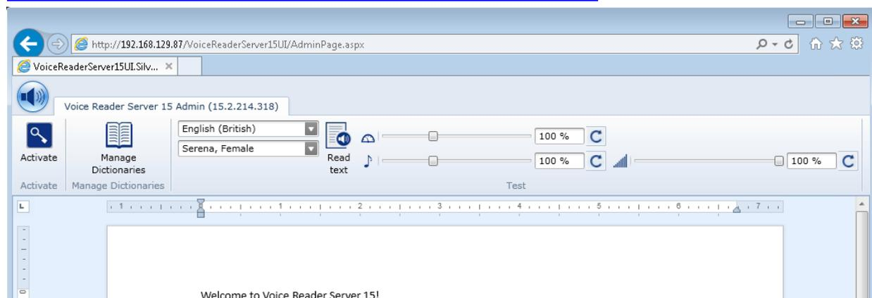
You can enter the desired text into the text box. The “Read text” button will start the text-to-speech process for simple reading. In the boxes for language and voice you can choose between the installed components. Use the slider bar to change the settings for speed, pitch or volume. The reset buttons will change the values to default.
